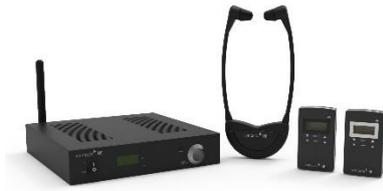
With a range of up to 150m, the RF-TX1 portable transmitter offered enough power for even the largest of the rooms in this project. As the RF systems can easily be channel swapped, multiple receivers could be used in the conference room if necessary. This feature delivered an ideal solution for the 18-room installation site.
