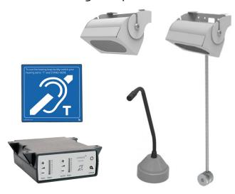
The STS-K062 Window Intercom System features a screen mounted microphone for the customer side, overhead speakers for the customer and staff sides and a round base staff microphone along with a above the counter hearing loop aerial. The system provides assistance for clear communication where normal speech is impaired by use of glass, a security screen or other similar barriers.
