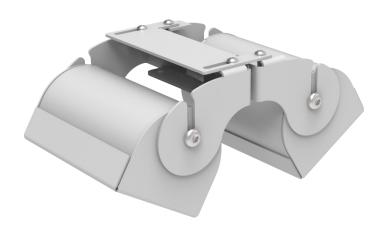
The STS-S23-BRKT-C Dual Clamping Bracket allows for two STS-S23 Overhead Speakers to be adhered to a freestanding glass or safety partition and similar screens where the top of the glass is exposed. The clamp is adjustable between 2-20mm to accommodate a range of glass thicknesses.
